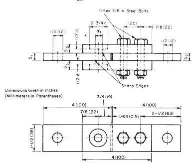
d = nominal diameter of specimen (rivet, wire, or machined specimen),
